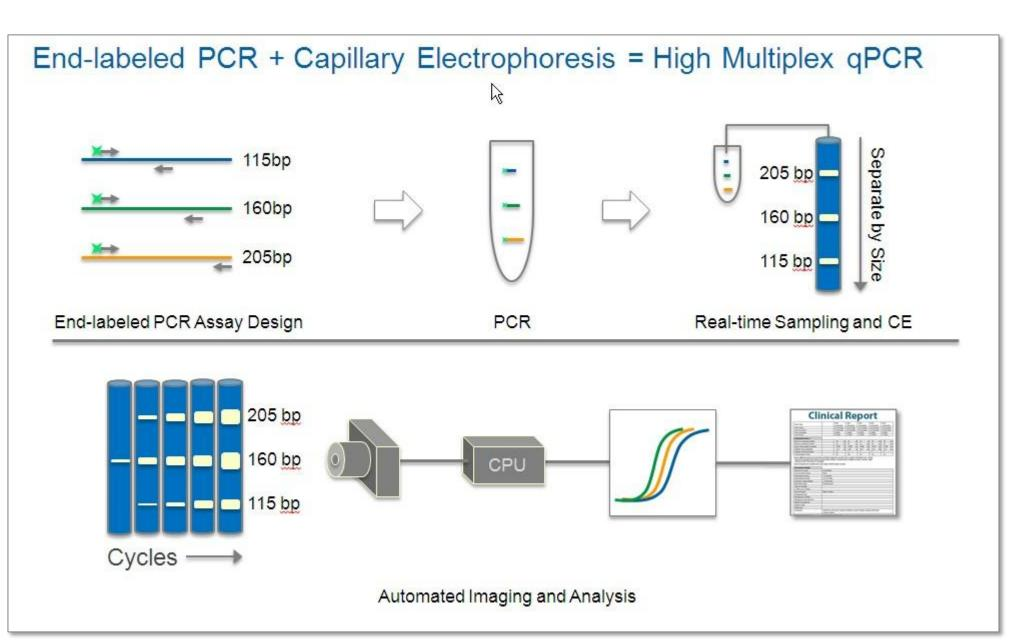
Figure 2. Principles of the multiplex real-time PCR detection on the ICE Plex System
